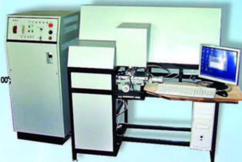
Apparatus for laser marking of gems and jewels
